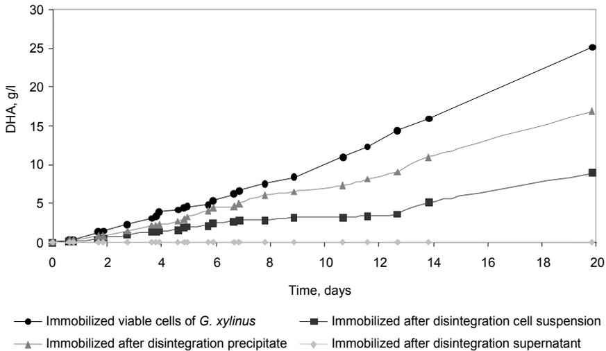
Fig. 2. Changes in DHA concentration in the production medium with the initial glycerol content of 30 g/l as affected by the time of biotransformation and type of immobilizate applied
