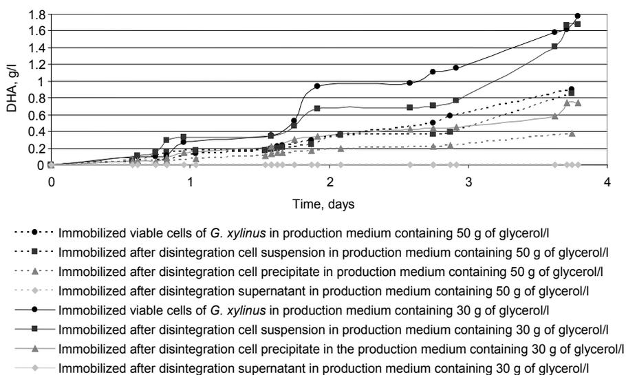
Fig. 1. Effect of glycerol content in the production medium and type of immobilizate on changes in DHA concentration during biotransformation
