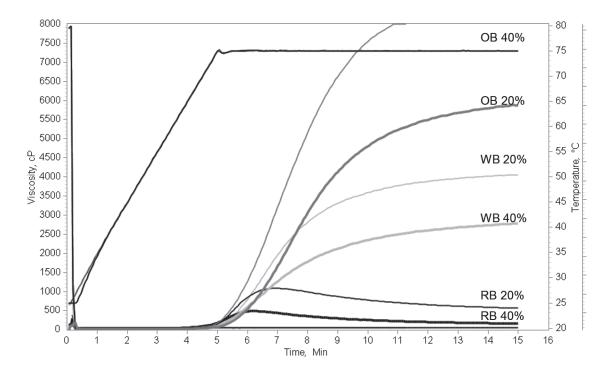
**Fig. 1.** Comparison of paste profiles of raw material blends according to Critical Paste Test: OB - oat bran, WB - wheat bran, RB - rye bran
