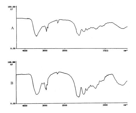
Fig. 4. IR Spectra of: A – collagen, B – elastin Rys. 4. Wimdma IR: A – kolagen, B – elastyna
