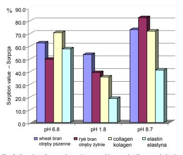
Fig. 2. Sorption of copper by various cereal bran and collagen and elastin preparations
