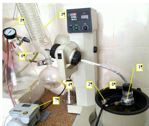
Fig. 1. Vacuum evaporator for massecuite boiling
