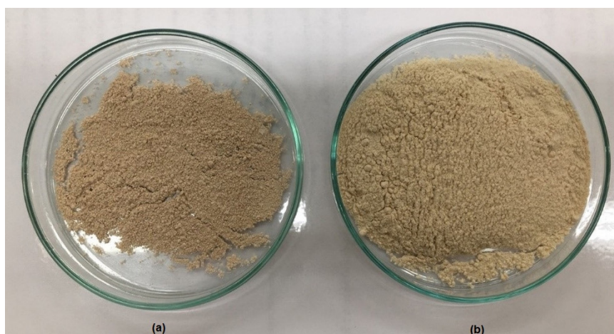
Fig. 1. Dried pectin: a – dried pectin (banana peel) extracted by UAE, b – dried commercial (citrus) pectin; \Delta E value or total colour difference between a and b was 6.68
